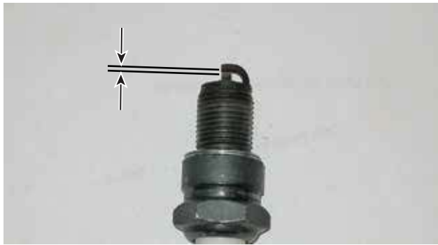
Figure 37 – Spark Plug Gap Requirements
