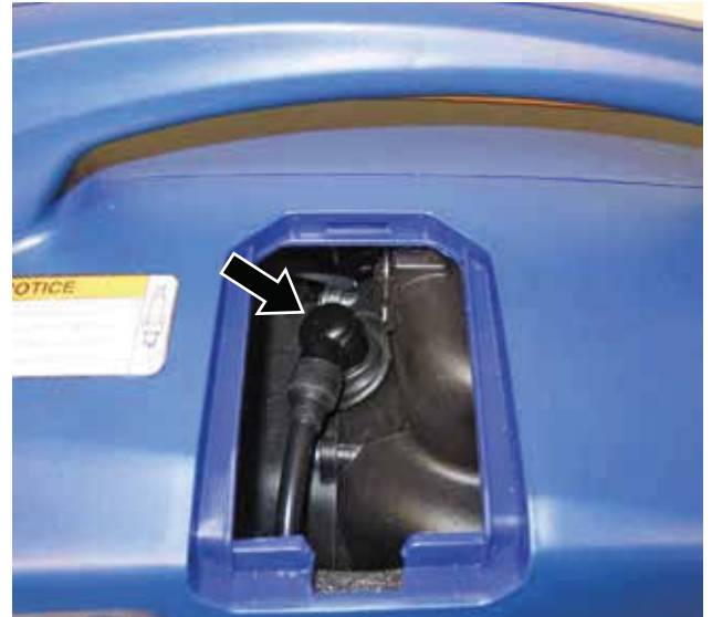
Figure 35 – Removal of Spark Plug Boot (WH1000i Shown)
