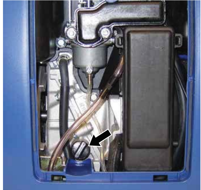
Figure 16 – Oil Fill/Drain Plug (WH1000i Shown)
