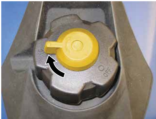
Figure 21 – Fuel Tank Vent
